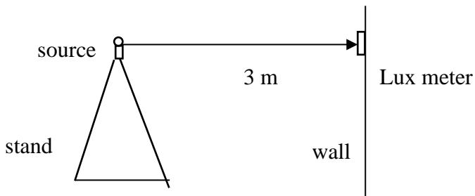
3. The room light is switched off. The normal supply is terminated by pulling the plug and the emergency light is automatically turned on.
