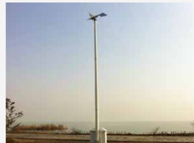
DM-1500 grid-tie system with 10.4m hydraulic tower installation - Sweden 2012
