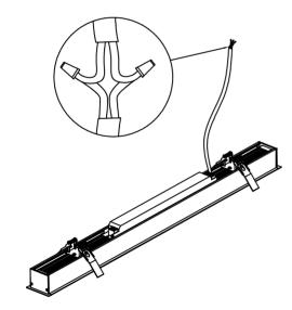
3. Use wire fixing connectors to connect luminaires with AC.
