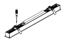
$2. Use \ screwholder \ to \ fix \ the \ spring \ brackets \ at \ the \ back \ of \ luminaire.$
