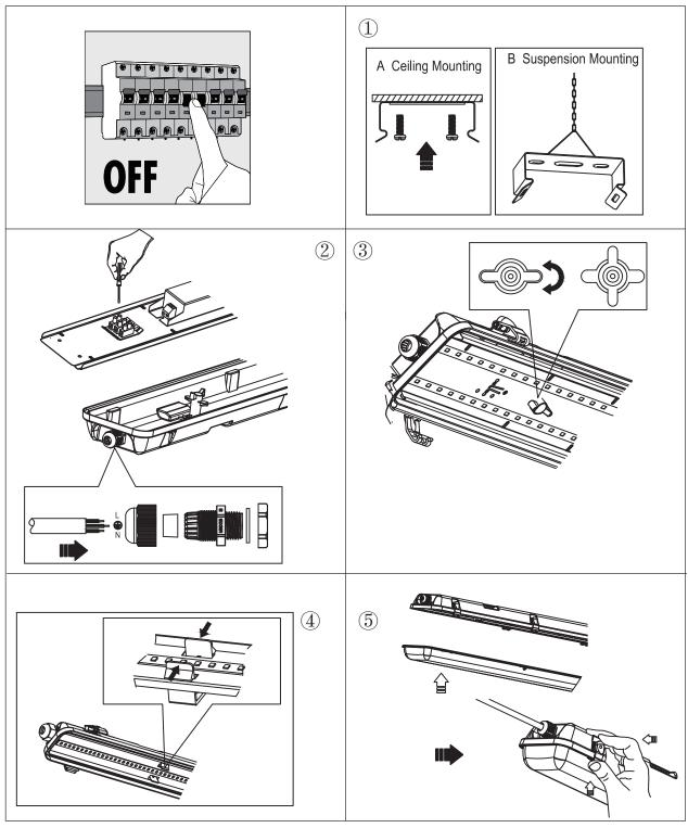
Remark: The fixture must be properly grounded to avoid accidental power leakage and electric shock.
