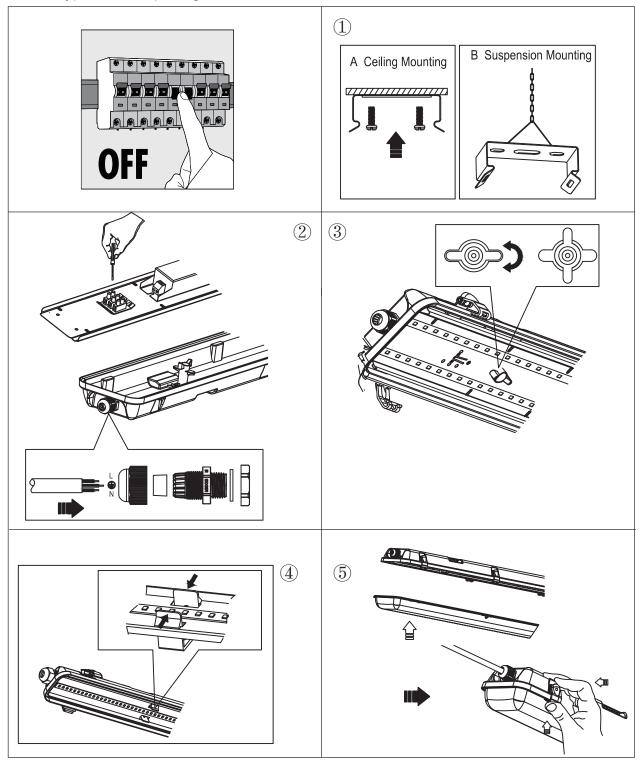
Remark: The fixture must be properly grounded to avoid accidental power leakage and electric shock. The fixture must be installed by a qualified electrician. Before installing be sure to turn the power off. \*For more details, refer to the BAWATY data sheet.
