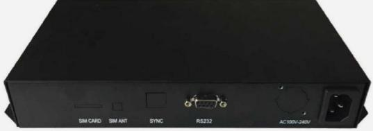
The CARIDE converter converts RS232 protocol commands into TCP/IP protocol commands, supporting animation segment selection, animation playback speed, overall brightness adjustment of the fixture, and white balance adjustment of the fixture.
