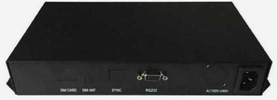
The CARIDE converter converts RS232 protocol commands into TCP/IP protocol commands, supporting animation segment selection, animation playback speed, overall brightness adjustment of the fixture, and white balance adjustment of the fixture.
