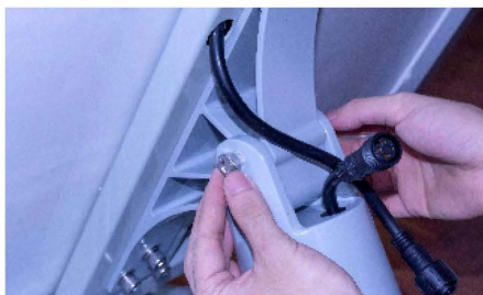
4.Mount the Vertical Bracket Module(in step3) into the Horizontal Bracket, keep the Vertical Bracket Module backside(with 3x screws) facing toward the light, tighten the bottom screw first and then the others after adjusting the Solar Panel vertically
