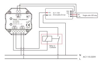
Note: We recommend the number of LED drivers connected to 0/1-10V dimmer does not exceed 5 pieces, The maximum length of the wires from dimmer to LED driver should be no more than 15 meters.
